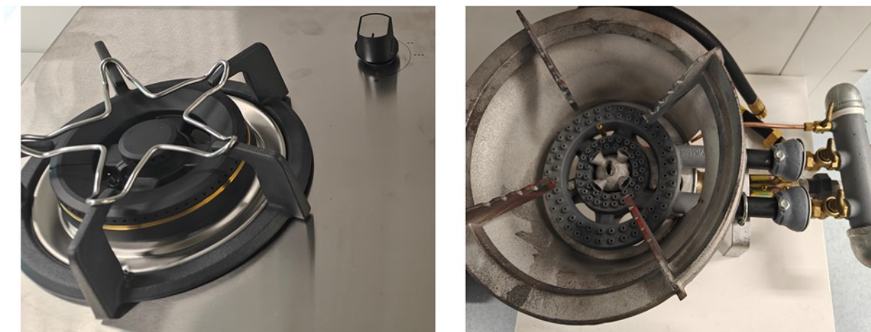
Figure 3.1: Cooking stoves used in the experiment. Left: Residential stove commonly used in households in Singapore. Right: Commercial stove typically used in food courts and hawker centers in Singapore.
